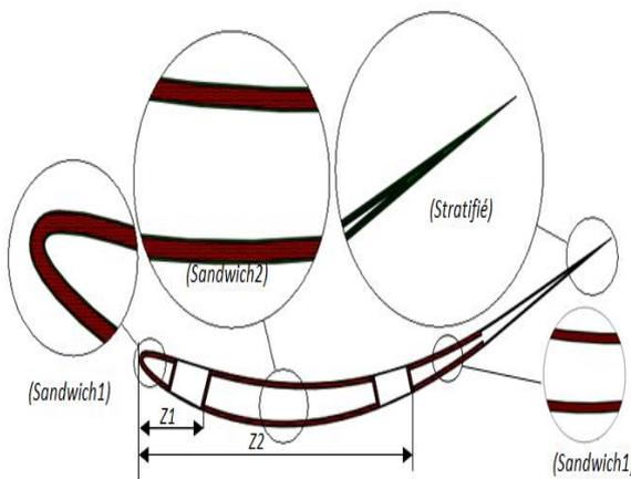
(a) Final iteration using the maximum deflection and the Hashin failure criteria
