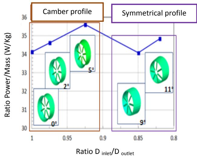
(b) Duct ratio <power/Mass> versus < $D_{inlet}/D_{outlet}$ >
