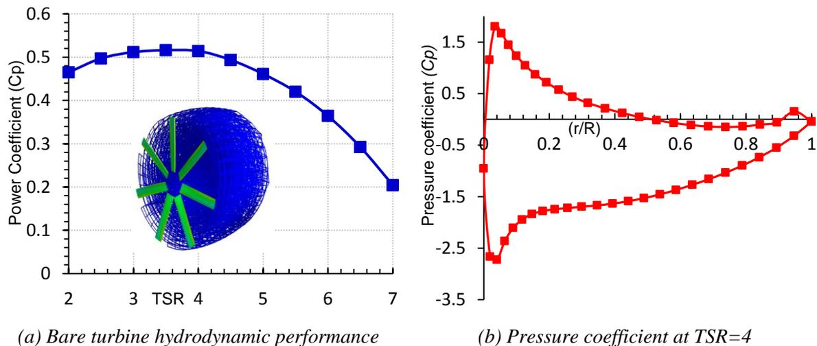
Figure 1: Hydrodynamic design of the bare turbine
