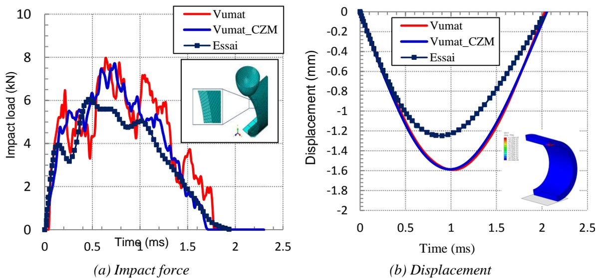
Figure 4: Comparison of experimental data (Essai) and numerical results (Vumat\_CZM) under impact energy of 5.20 J ( $V=2.5$  m/s)
