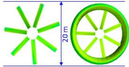
(b) Bare and ducted tidal turbine at the same overall cross section of 20m
