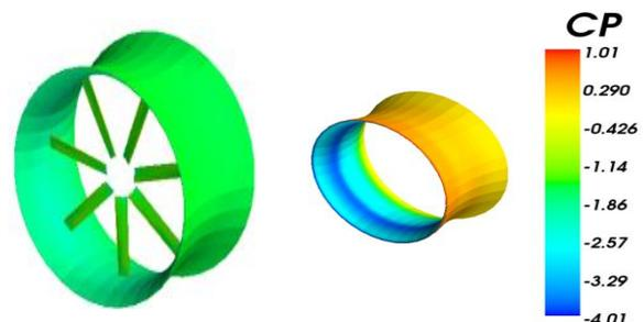
(c) Final ducted turbine design (left) and hydrodynamic pressure (right)
