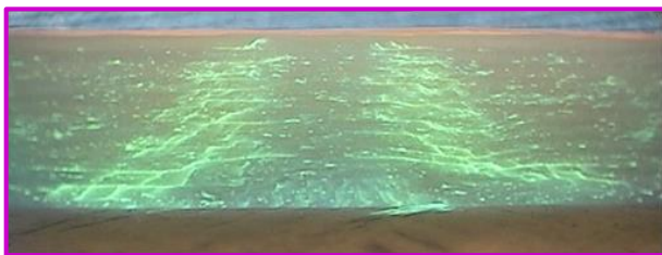
Axial section through damaged cylinder wall using UV lighting
